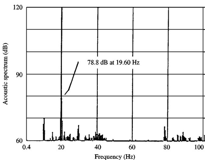
Figure 6. Acoustic spectrum of two parallel non-interacting air-jets issuing from 25 mm diameter tubes; obtained with 12 averages. Measured at 1 m distance in free space. Reynolds number  $Re = 100\,000$ .
