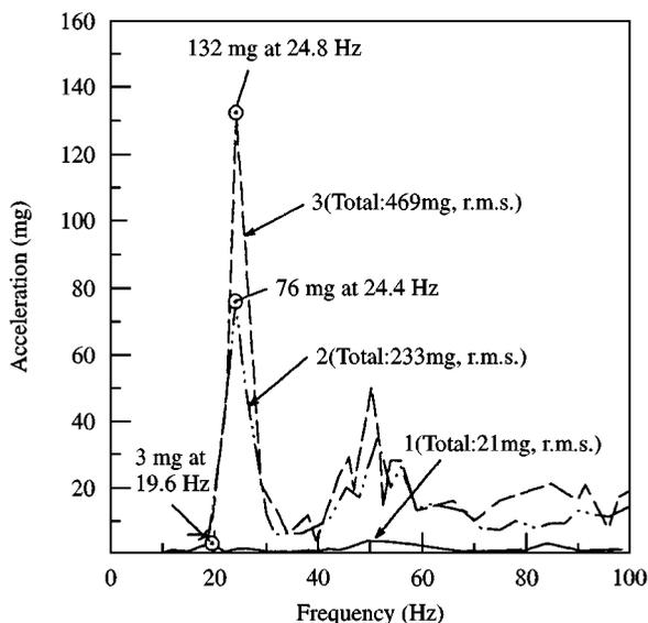
Figure 2. Vibration acceleration spectra taken at mill casing at door of spring plunger: 1, no vibration at  $\sim 70\%$  load; 2, vibration at  $\sim 40\%$  load; 3, severe vibration at  $\sim 30\%$  load; (mill original configuration).
