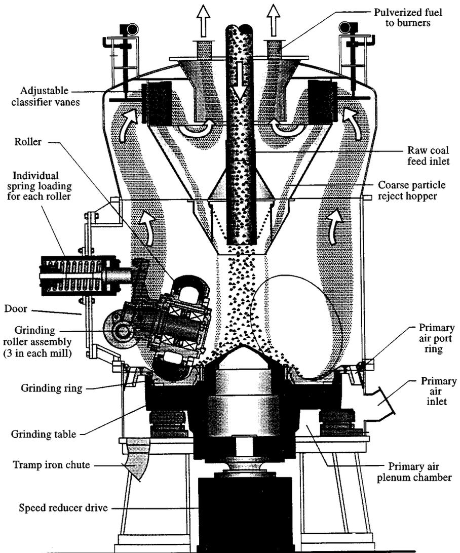
Figure 1. General arrangement of coal pulverizer (MBF-type pulverizer by Foster Wheeler).
