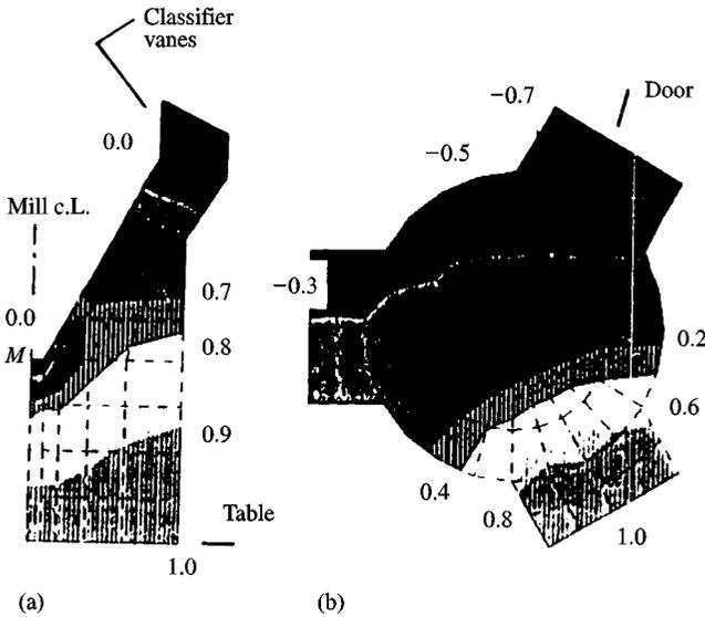
Figure 4. Acoustic pressure modes inside mill casing in mill grinding zone: (a) fundamental quarterwave vertical mode at frequency of 24.7 Hz; (b) second horizontal (transverse) mode at frequency of 52.2 Hz.
