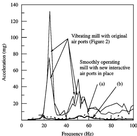
Figure 11. Comparison of mill vibratory and nonvibratory conditions with the original and new interactive air ports in place, respectively. Vibration acceleration spectra taken at door of spring plunger. *Non-vibratory condition:* (a) at 35% load, (b) at 92% load. Maximum vibratory acceleration: 5 mg r.m.s.; maximum total vibratory displacement: 8  $\mu$ m, r.m.s.
