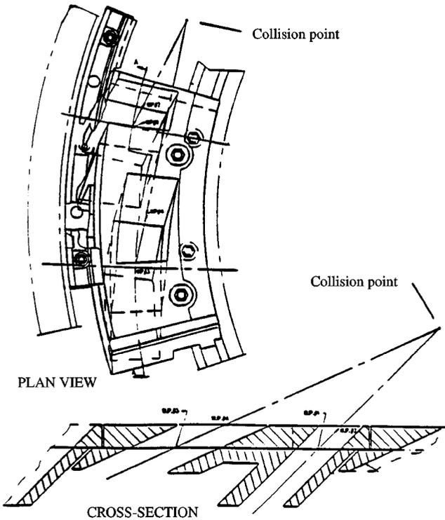
Figure 10. New design of mill air ports with air-jet interaction (collision) features incorporated.
