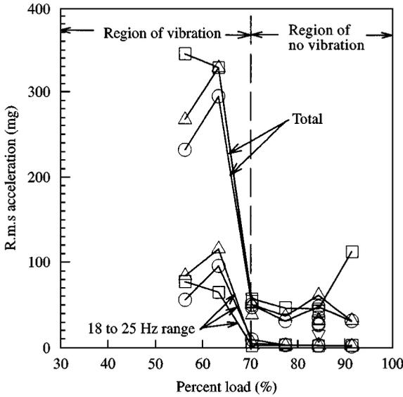
Figure 3. Typical vibration versus load relationship showing regions of no vibration and vibration. Acceleration readings taken at mill casing at three locations at door of spring plunger; (mill original configuration).
