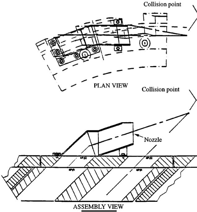
Figure 9. Nozzles attached to air ports of mill redirecting air-flow. Nozzles attached to every other air port to produce collision of air-jets; (test arrangement).
