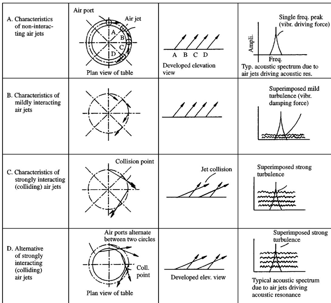
Figure 8. Schematic arrangement and acoustic vibration potential of non-interacting, mildly interacting and strongly interacting air-jets issuing from air ports (sample configurations).
