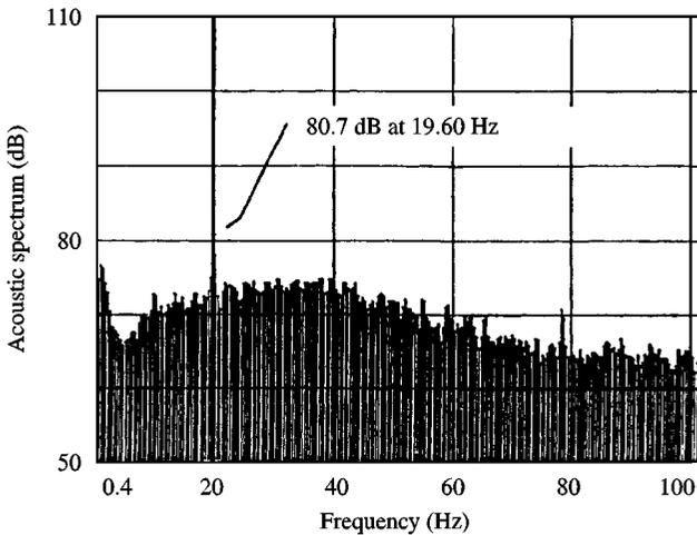
Figure 7. Acoustic spectrum of two intersecting (colliding) air-jets issuing from 25 mm diameter tubes; obtained with 30 averages. Measured at 1 m distance in free space. Reynolds number  $Re = 100000$ .
