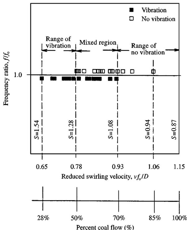
Figure 5. Map showing cases of vibration and no vibration versus coal flow and reduced swirling velocity. Interpretation of test results based on coincidence of swirl-induced excitation frequency  $f$  with fundamental quarterwave acoustic frequency  $f_0$ ; (mill original configuration).
